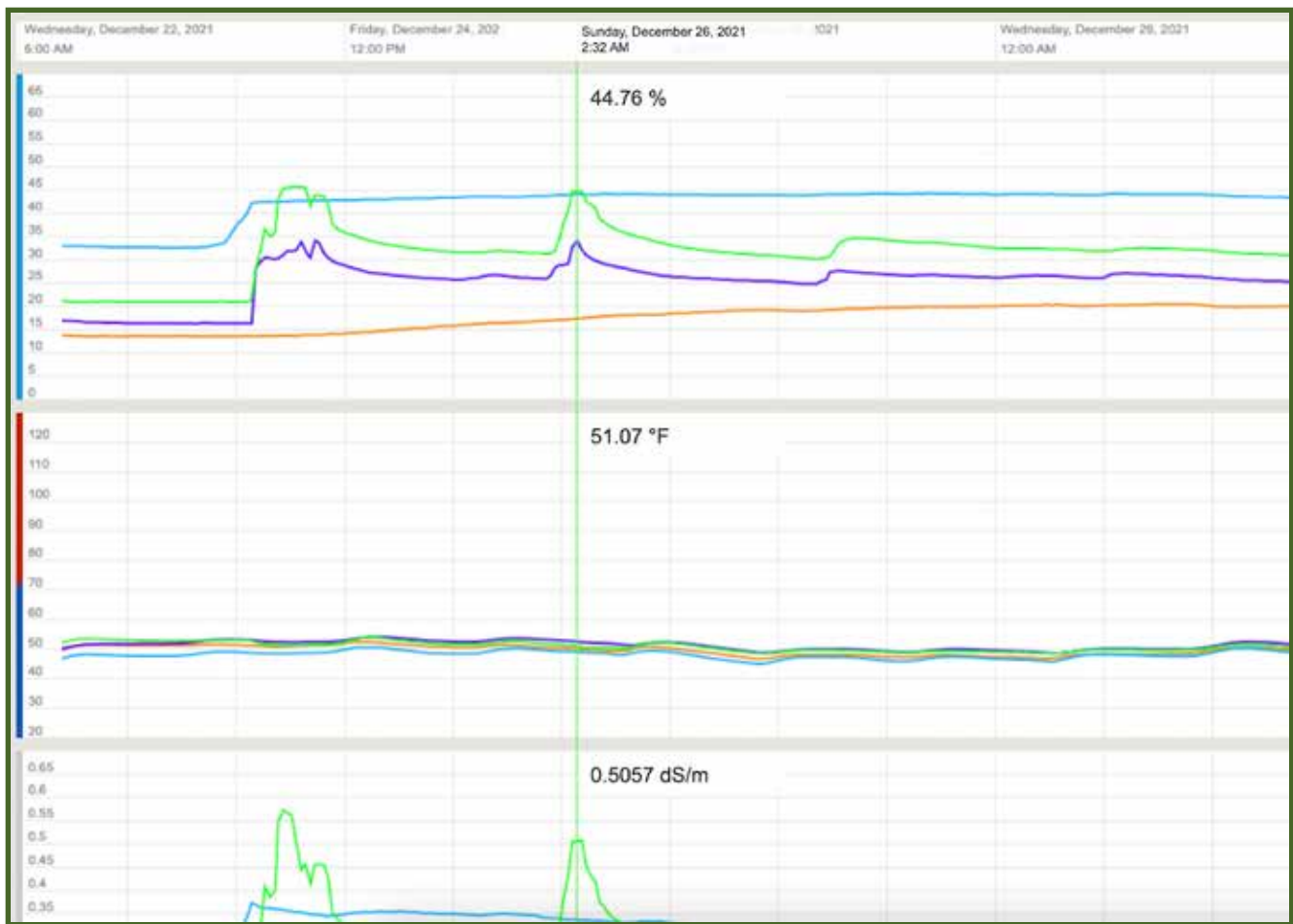
Web based application that makes sense of sensor data and can chart soil moisture, salinity, and temperature levels.
