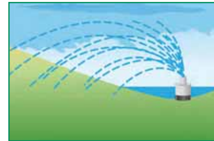
Sprinkler without check valve
