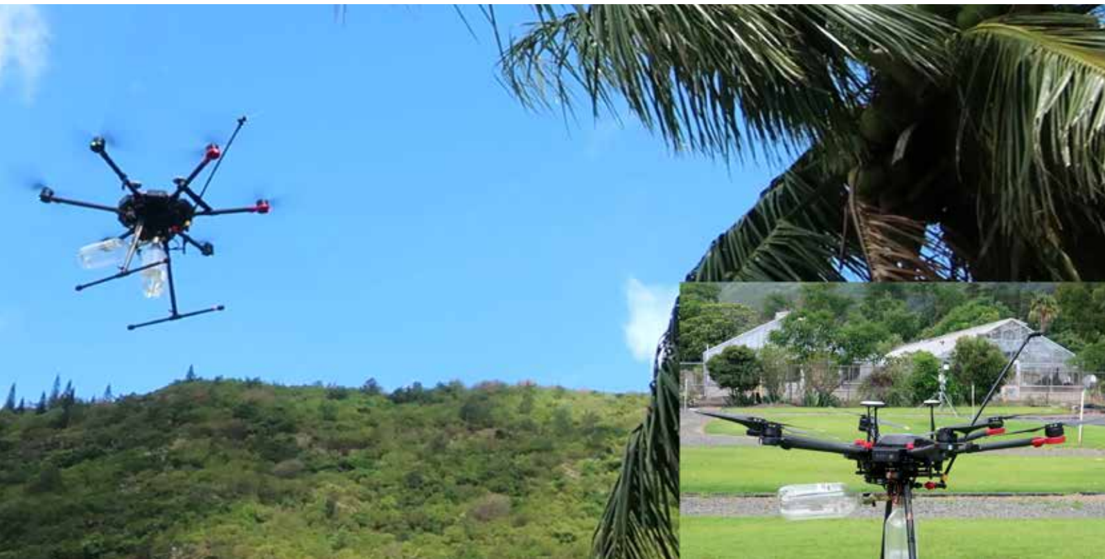
A prototype research drone fitted with liquid tank and CO2 compress gas reservoir commissioned to apply spray solutions to coconuts and other large trees in the landscape setting (inset photo). The flying sprayer was designed to spot apply a stream of liquid to specific targets in the coconut crown.
